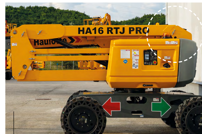
BOOM PROTECTED by the counterweight frame
