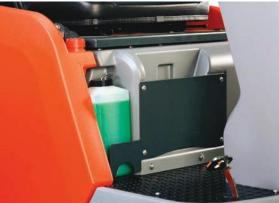
The on-board dosing system is completely integrated in the machine design and ensures that optimum quantities of cleaning detergents are added, depending on the amount of water used.
