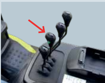
VMS activation switch on the mechanical hydraulic lever
