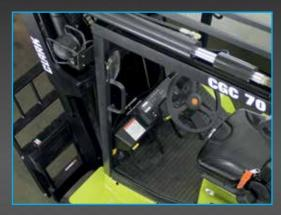
The interior of the generously designed operator's workplace offers the driver sufficient headroom and legroom. The driver can enter and exit comfortably via a large step. Handles on both sides of the truck increase safety. The steering column is tiltable and can be adjusted individually.
