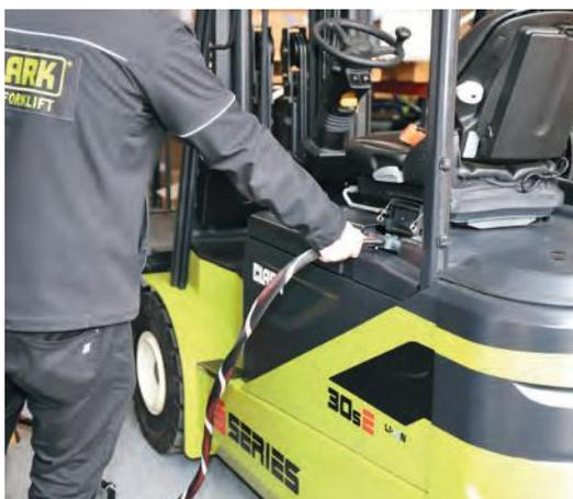
Recharging the Li-ion battery is possible from a standing position for the driver is possible without having to open the battery hood.
